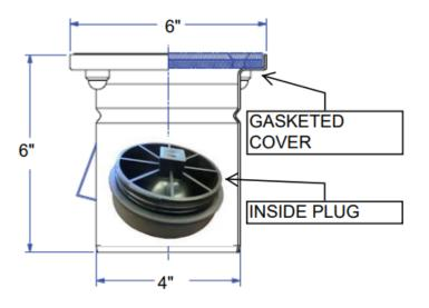
**Engineering Specification:** 304 STAINLESS STEEL & SMOOTH HEAVY DUTY SOLID GASKETED COVER. INSIDE PLUG Meets The ASME A112.6.3 requirements.
